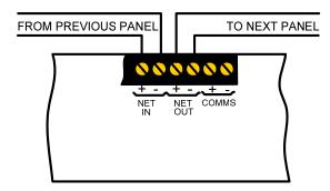
The network connection must come into each panel on the "Network In" terminals and go to the next panel on the "Network Out" terminals, returning to the first panel "In" from the last panel "Out" terminals.
