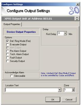
Control of outputs uses the same philosophy as that described for inputs, i.e. all outputs are treated the same, whether they are loop controlled relays, loop sounders, sounder controllers, panel sounder outputs, panel programmable relays, remote I/O board outputs or the panel mounted programmable LED indicators.
