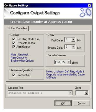
**NOTE:** If a loop sounder is controlled by a cause and effect operation, then the Tech Alarm tone will be used when the sounder is energised.
