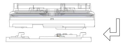
To release, push Release Tool into holes in rim of sounder unit and slide the product in the reverse direction.
