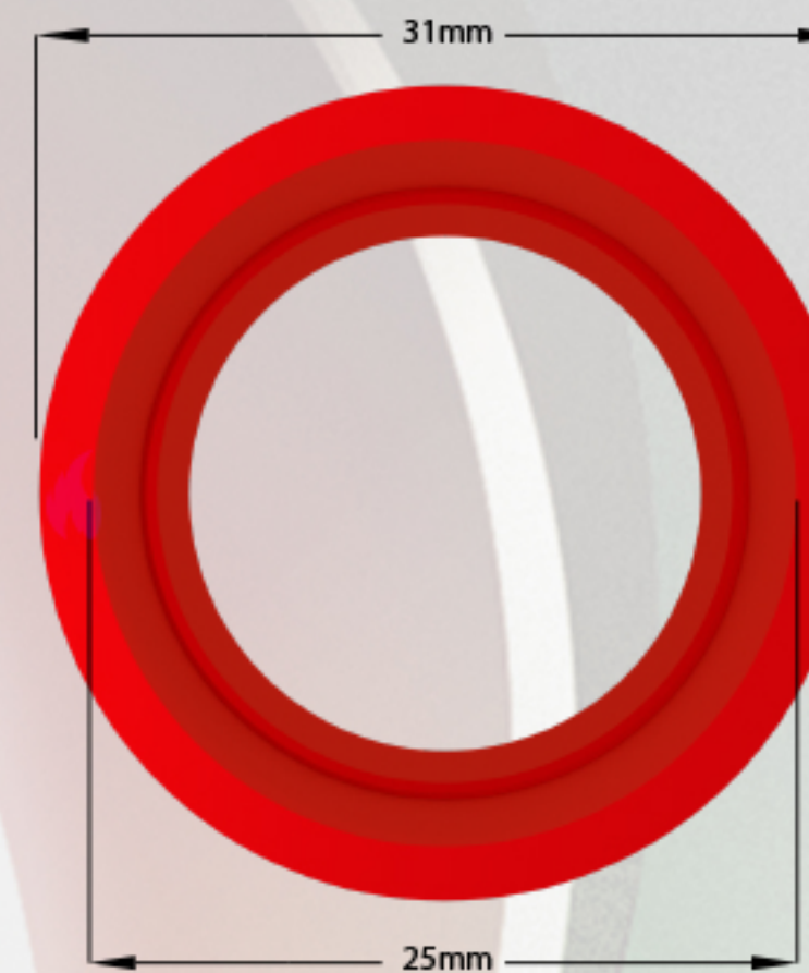
Jointing Socket Front Elevation
