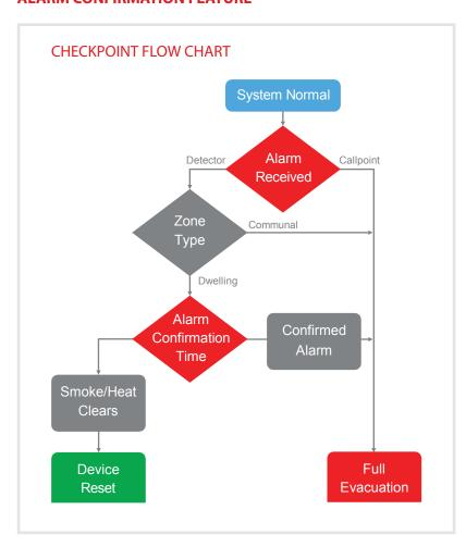
Using the built-in alarm confirmation feature, until an alarm has been confirmed within an individual area, only that area is evacuated. At the same time, if an alarm is triggered in a common area, the device initiates a full alarm evacuating all surrounding areas. This unique panel feature is vital where two- stage alarms are required.
