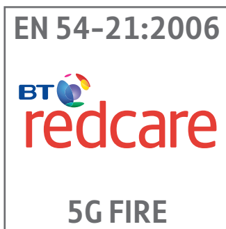
Fig 2. For fire installations apply a label to the outside of the STU enclosure.
