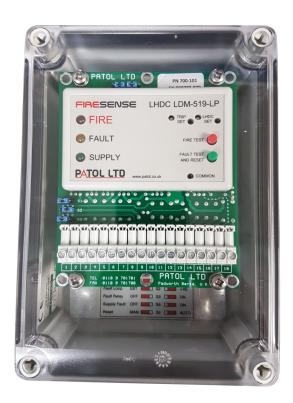
The module is designed to monitor a zonal length of Analogue Cable for both an elevated temperature (Fire) condition, and Fault Status (Open & Short Circuit).
