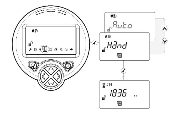
If it is not possible to see the LASER because of the installation environment (for example, if you cannot see the Reflector from the System Controller or there is high ambient light) then use 'Hand' Alignment. This option displays the signal strength value returned by the Detector, and allows the user to move the beam
