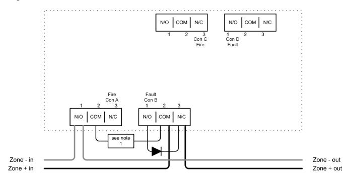
Note 1 – This component is the Fire Resistor. Its value is specified by the FCP manufacturer, and is not supplied with the System Controller. For U.S. installations it is typically a short circuit.
