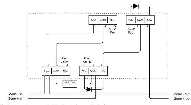
Two Detectors connected to Controller:
