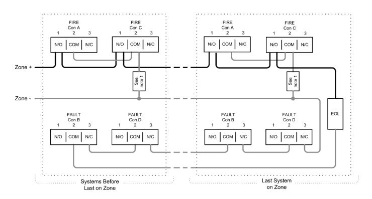
Note 1 – This component is the Fire Resistor. Its value is specified by the FCP manufacturer, and is not supplied with the System Controller. For U.S. installations it is typically a short circuit.
