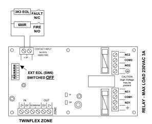
For use as a fault monitored input, connect to input as shown above, **remembering to set the External EOL switch to OFF**.
