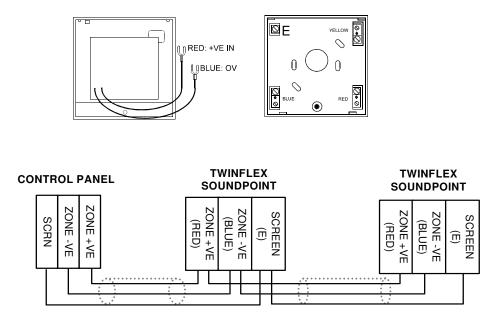
Twinflex Soundpoints can be mixed on the same zone as other types of Twinflex device (eg. Twinflex Multipoint Detectors). The above diagram shows how to make the zone positive, zone negative and screen connections between the control panel and Twinflex Soundpoints. Refer to the instruction leaflets supplied with other Twinflex devices for their equivalent wiring/terminal labelling details.
