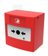
When activated, a plastic 'flag' is displayed in the window of the unit; the supplied key will reset the flag and unit. Supplied with back box.
