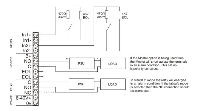
When the system is operating in the test mode, depending on the settings, the relay and mosfet operation will not operate, however the inputs will still remain enabled.
