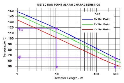
LHDC Interface Modules are equipped with sensitivity / trip adjustments. The graphs show three typical settings; 1V, 2V and 3V.
