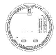
The Loop IN +ve (positive) and the Loop OUT +ve (positive) connections are split within the module. For cable continuity readings at the commissioning stage they must be temporarily removed and connected through. Please remember that all high voltage testing must be carried out before the installation of the electronics, otherwise the electronics will be damaged. Please also note that the SCRN terminal should only be connected to the loop screen and NOT the building earth.
