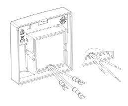
Care should be taken when terminating devices to ensure all cables are correctly sleeved and connections are secure. Improper connections will prevent a system from responding properly in the event of a fire.
