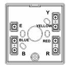
The Loop +ve (positive) IN and the Loop +ve (positive) OUT connections are split within the module. For cable continuity readings at the commissioning stage they must be temporarily removed and connected through. Please remember that all high voltage testing must be carried out before the installation of the electronics, otherwise the electronics will be damaged. Please also note that the E terminal should only be connected to the loop screen and NOT to the building earth.
