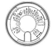
The Loop +ve (positive) IN and the Loop +ve (positive) OUT connections are automatically joined together (short circuit) by a spring arm between terminals 2 and 3 until the detector is installed. This allows for cable continuity readings at the commissioning stage.
