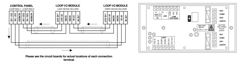
Before installing the module remember to note the serial number of the device (located on the rear of the unit) on to your drawings or configuration sheets to enable you to prove its location later. The address allocation for the device is carried out automatically by the control panel whilst in initialisation mode, so addresses do not need to be set manually. See the system Installation and Operating Instructions for further details.
