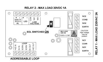
For use as a simple 'change-over' relay output, connect as shown on the left, **remembering to set the EOL** (end of line) switch to ON.
