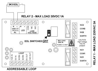
For use as a 'change-over' relay output with fault monitoring, connect as shown on the right, **remembering to set the EOL (end of line) switch to OFF**, and to use a volt free fault contact to break the EOL circuit in order to generate a fault condition.
